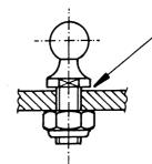
Gap generated by unscrewing of the ball end or wear out of the fitting material.
