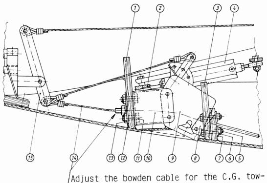
Adjust the bowden cable for the C.G. towing hook in such a way that both towing hooks open completely at the same time when actuated!
