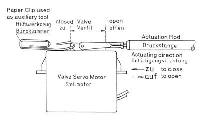
Fig. 2.4-3 Valve Operation
