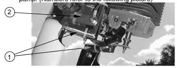
3. Check for proper placement and lock of the electric line connector at the front end of the engine bay.
