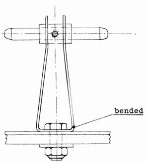
3. Mount new support with new screws and nuts. Notice: No bearing thread, cut thread exactly.
