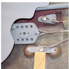
2.) The handle for the towing cable release in the front and rear seat is relocated to ease its operation in case of limited mobility of the legs.
