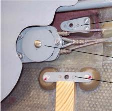
Anchor point for disconnected cable of the front pedal.
