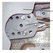
Connection plate for cables of rudder pedals with demounted lock washer. The removable connection bolts are visible.
