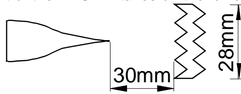
Fig. 4 - Zig-Zag-Tape in front of the NACA-Intakes on the lower wing surface
