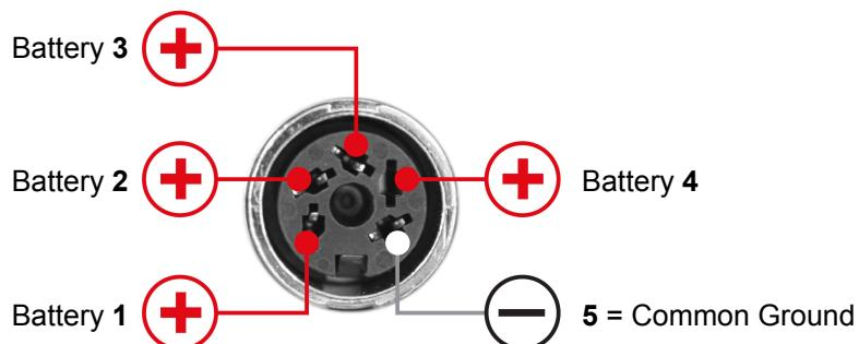
To facilitate battery charging, Alexander Schleicher GmbH and Co. offers adapter cables for connecting a charging device to the charging socket in the panel. The adapter cable connector is labelled to ensure that the charger is connected to the correct poles of the charging socket.
