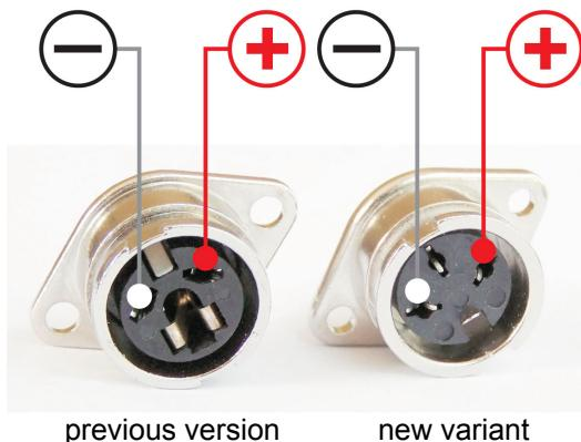
**Note:** When replacing the charging socket, the corresponding plug must be also replaced, because on the new variant the position of the pins have been changed.
