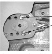
Connection plate for cables of rudder pedals with demounted lock washer. The removable connection bolts are visible.
