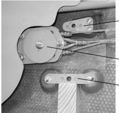
Anchor point for disconnected cable of the front pedal.
