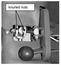
The adjusting screw for the cable tension of the rudder hand control system is located in the front of the control column and besides of the pedal adjustment. This is for the **fine adjustment** of the cable tension during the Pre Flight Check.
