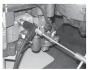
Now the spark plug can be unscrewed using a socket spanner A/F 16
