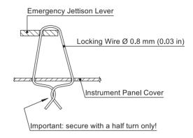
Never twist the locking wire more than a half turn, as this will prevent the operation of the emergency jettison! In case of any doubt test the operation of the emergency jettison with the locking wire installed and install a new locking wire later in the same way.
