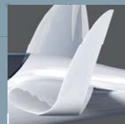
CFD optimized winglets for best handling qualities.
