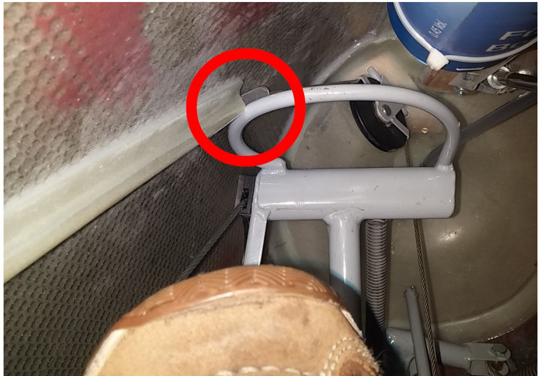
Fig. 1: Possible jamming of the rudder pedal with the cable guide of the release mechanism cable
