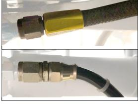
Brake hoses of the **old type** made from rubber material, identifiable by the shown fitting shape and the textile fabric wrapping of the hose.
