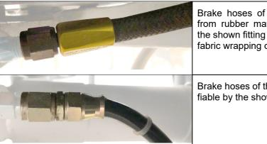
Brake hoses of the **old type** made from rubber material, identifiable by the shown fitting shape and the textile fabric wrapping of the hose.
