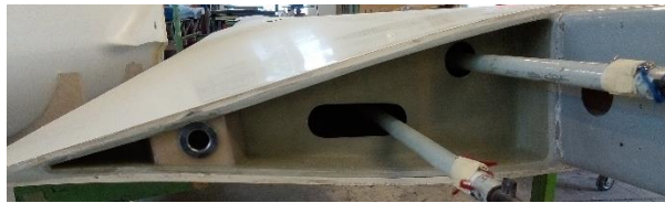
Finally bonded new GFRP rib.
