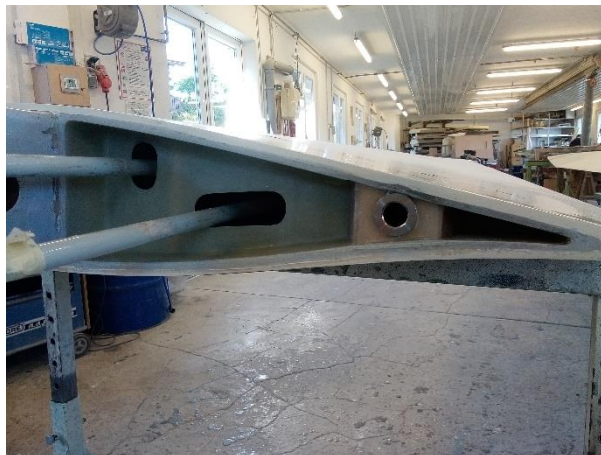
Final rearward GFRP rib prior to preserving.
