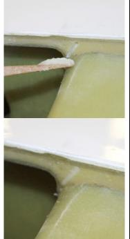
Fill the crack with bonding cement (refer to section "Material and Drawings") and smooth down.
