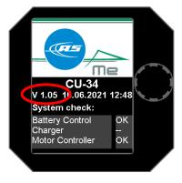
The current software-version must comply with one of the approved versions listed in the following Table 1. If this is not the case, the software must be updated until the next scheduled maintenance of the propulsion system.
