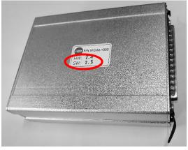
The current software-version must comply with one of the approved versions listed in the following Table 2. If this is not the case, the software must be updated until the next scheduled maintenance of the propulsion system. When updating the software on the battery-manager note the new software version on the label!
