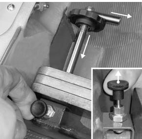
Position the trim plates in front of the mounting support and slide the guide rod through the plates. The handle of the guide rod must be horizontal and pointing outwards.
