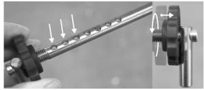
Check snap-in holes at guide rod for soiling. Turn back the clamping wheel completely.
