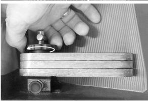
Finally fix the trim plates with the clamping wheel.
