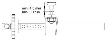
Furthermore, all components must to be checked for wear. See also section 7.10 in the Flight Manual.
