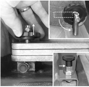
Now turn the handle of the guide rod vertical downwards and pull back the guide rod to the next locking position.
