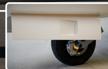
Standard Absaughute zur Steigerung der Cockpitbelüftung cockpit air extractor for increased ventilation
